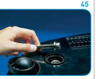
• Turn the appliance upside down (after having removed the lid and bucket and emptied the water in the refill tank), then use a screwdriver to remove the cover below.
