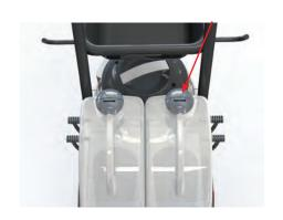
Pour 0,26 gal of tap water into the tank washing extraction. Connect the appliance to the mains and press button (C) on the display.
