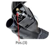
Check the O-rings on the connector for damage:
